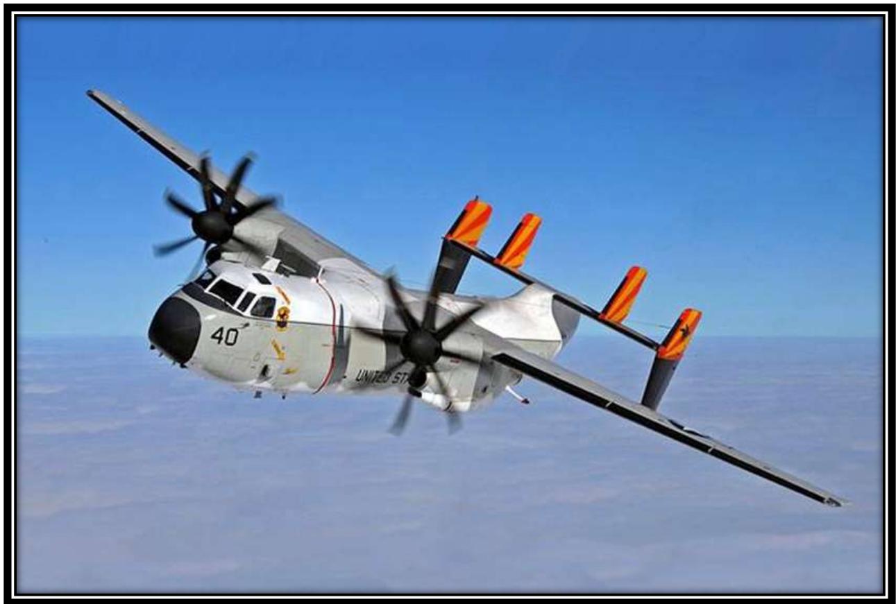
Photo 2. A Grumman C-2 Greyhound. The prime COD U. S. Navy aircraft since the mid-1960's.
