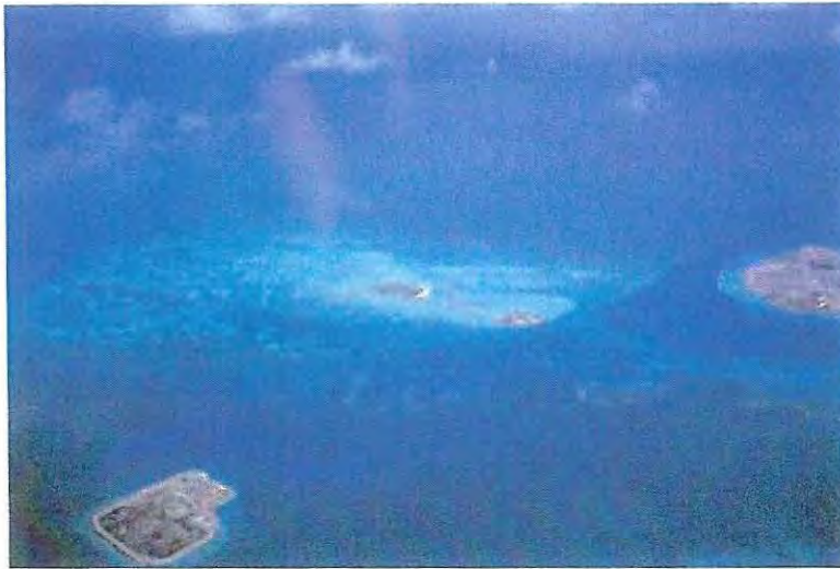
FIG. 17.7. Sand Island is in center, Johnston Island (partial) to right, North Island in foreground. The darker blue channel between Sand and Johnston was dredged from the reef to make a large ship channel and expand the islands. The coral carved from the rectangular basin adjacent North Island was crushed to create the artificial island
