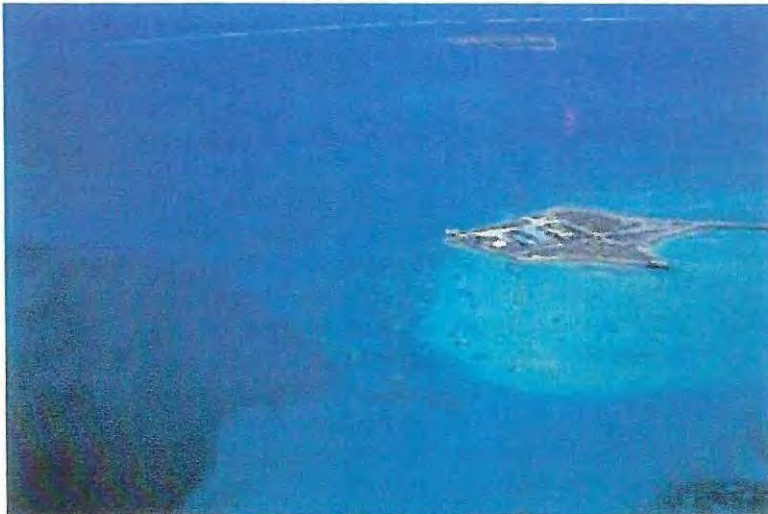
FIG. 17.9. This photo gives an interesting perspective of the dredged channel next to Sand Island. The dark blue channel is about 40ft (14 m) deep and was carved from reefs that were growing to the surface that still exist adjacent to the channel. The bright sandy area is very shallow sand flats (10ft, 3 m depth or less). The buildings were removed in 2001 and buried in place as a small hill (landfill). The north side of this west end of Sand Island is where most PCB contamination was found. Plutonium radiation was found on the south side. North Island is in background. The reticulated pattern of shallow lagoon reefs made boat travel a maze game
